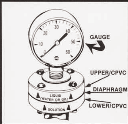
Threaded 1/4" for pressure gauge and 1/2" or 1" for line installation.
